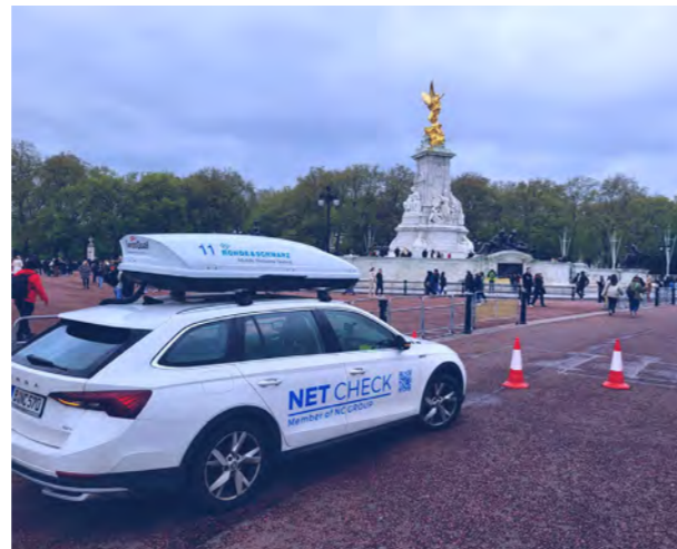
NET CHECK drive testing
